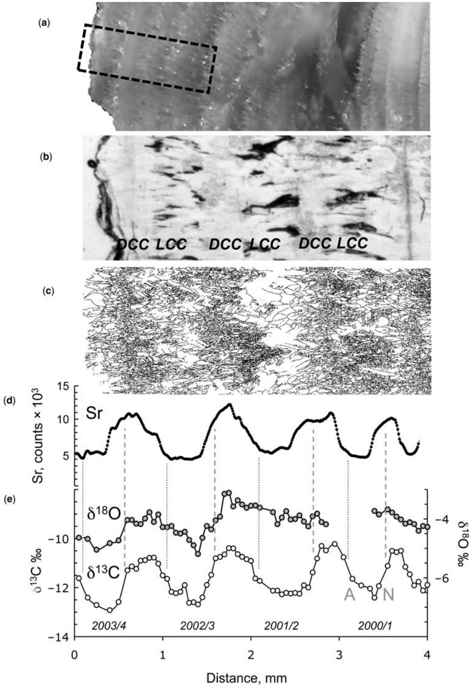
**Fig. 10.** Relationship between petrographic, trace element and stable isotope variations for laminae pairs growing over four years from 2000–2004 in Gib04a. (a) Macroscopic appearance of the uppermost portion of Gib04a. Active growth surface on left; width of image 11 mm and adapted from Matthey *et al.* (2008). (b) Area outlined in (a) prepared from facing slice as a thin section and viewed in plane polarized light. DCC, Dark compact calcite; LCC, light columnar
