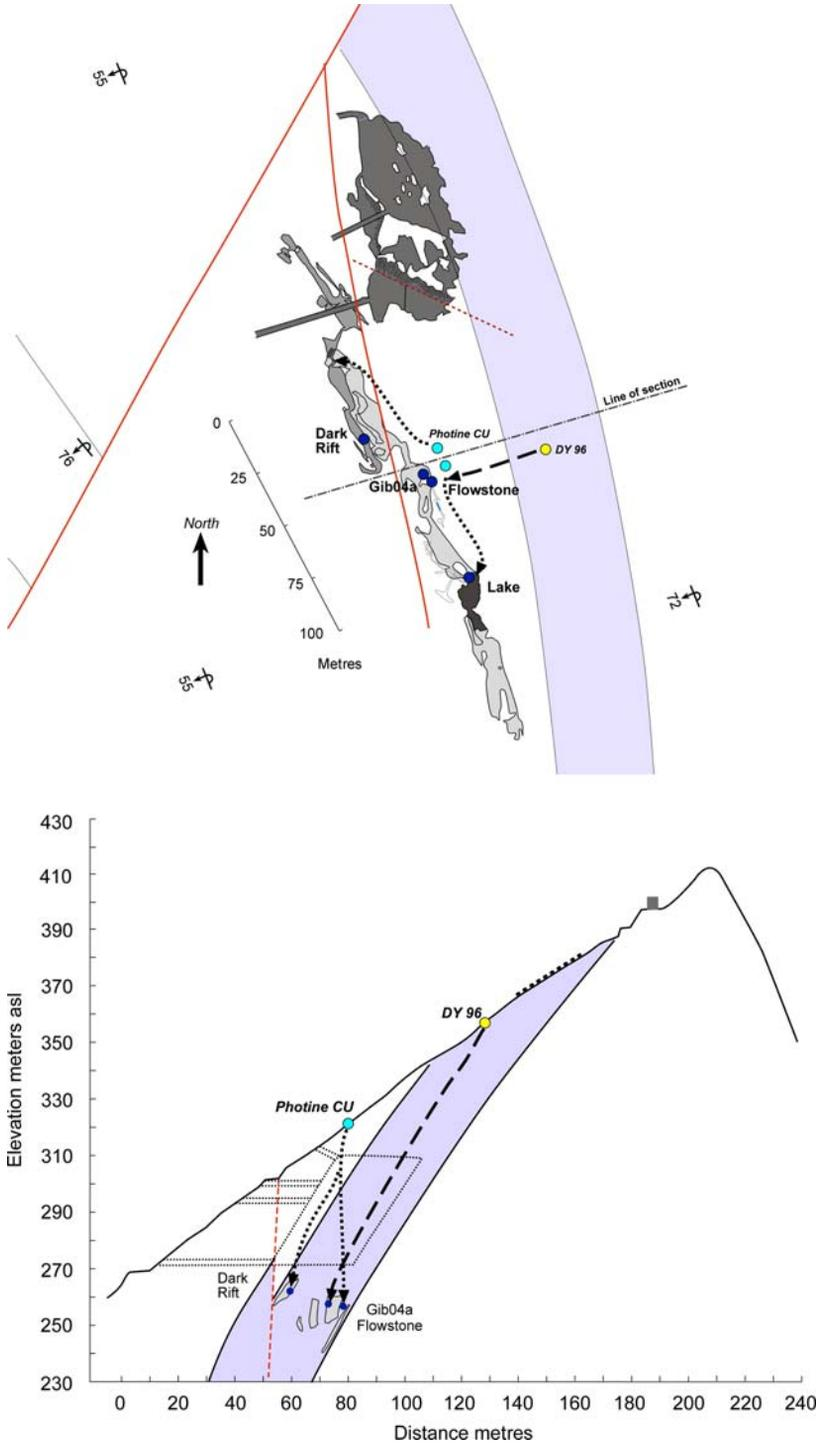
**Fig. 3.** Geological setting of St. Michaels Cave showing injection sites for the yellow dye DY96 (yellow) and blue dye Photine CU (blue) together with schematic flow pathways. Bedrock geology adapted from the map compiled by Rosenbaum & Rose (1991). Cave plan located relative to 1000 m UTM grid co-ordinates using data from a new line survey carried out in 2007.
