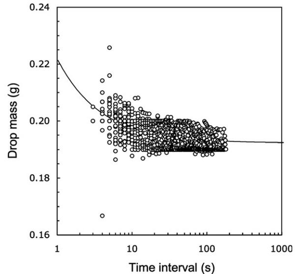
**Figure 6** Relationship between drop mass ( $r = 34$  mm) and supply flow rate, expressed as a function of interval between drops. The empirical relationship between drop interval and drop mass derived by Joos (1999) is fitted to the data. See text for discussion.
