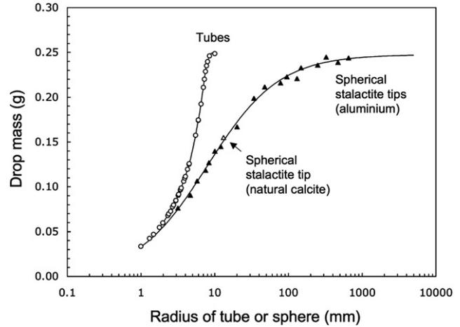
**Figure 4** Relationship between drop mass and radius of curvature of the detachment surface for aluminium (closed triangles) and natural calcite (open triangle) stalactite tips. Data for drop mass as a function of tube radius (Harkins and Brown, 1919) is shown for comparison.
