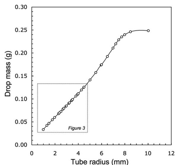
**Figure 1** Relationship between drop mass of water at 20 °C and radius of circular tubes (glass and brass) at drip intervals > 3 min using data from Harkins and Brown (1919).
