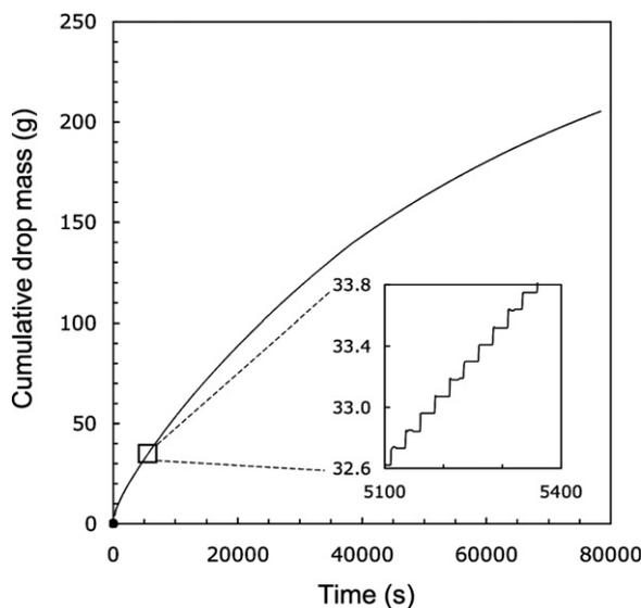
**Figure 5** Relationship between cumulative mass of drops falling from an artificial stalactite ( $r = 34$  mm), and time, measured for a decreasing water supply rate from a draining reservoir. Inset: enlarged portion of the main curve showing stepped increase from which drop volume and time interval can be inferred. See Discussion.
