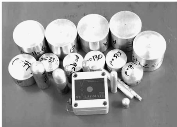
**Figure 2** An acoustic drip logger and artificial aluminium stalactite tips with radius of curvature ranging from 3.5 mm to 500 mm used in this study.
