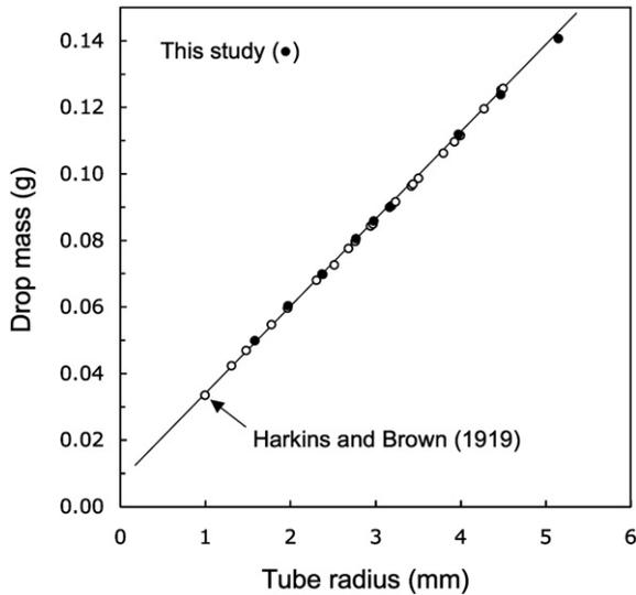
**Figure 3** Comparison of the relationship between tube radius and water drop mass measured in this study (closed circles) with data from Harkins and Brown (1919) (open circles and best fit straight line).
